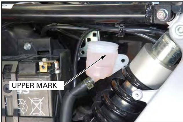
12. Bleed the pedal brake lines (rear master cylinder to rear caliper, then front calipers) in the following order:
