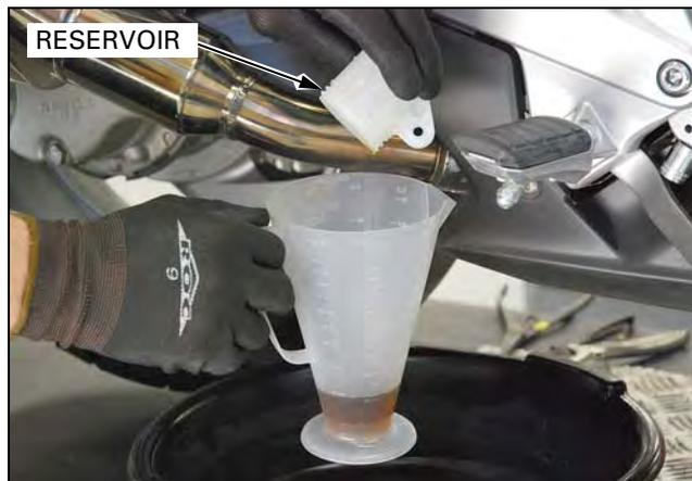
6. Using a suitable squeeze bottle and a 1/4 in OD x 12 in long hose, siphon the remaining brake fluid from the bottom of the reservoir hose as shown. This will ensure that very little brake fluid is spilled later.
