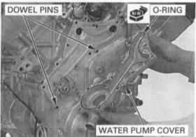
Install and tighten the water pump cover bolt.
