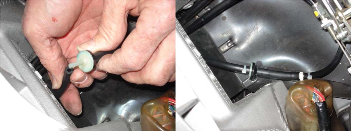
17. The control cable is connected to the bracket, and then connected to the lever via the chain. Shrink tubing is added over the coupling between the ball at the end of the cable and the chain.
