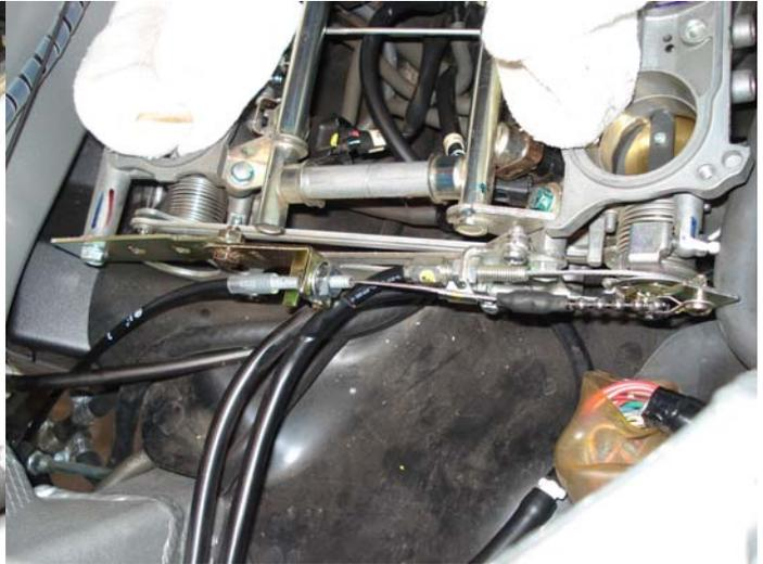
18. The Violet wire from the Audiovox cruise control is connected the Green/Yellow wire from the Red connector on the front right side of the bike. The Green/Yellow wire is on the rear (left) half of the Red connector. The wire was extracted from the connector and the Violet wire was soldered to it, and covered with shrink wrap.
