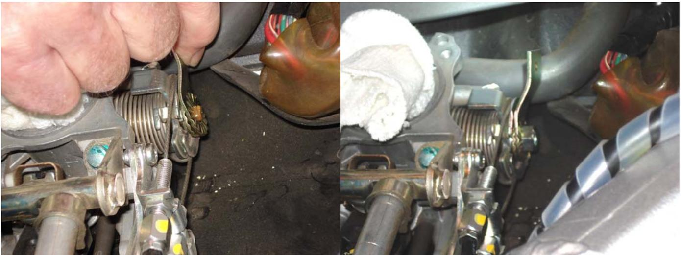
10. Install the opposing Audiovox bracket on the throttle body. One screw will need to be removed and re-installed thru the bracket.
