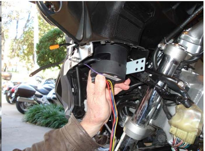
13. Zip ties were used to attach the control box the bike. Dry fit the panels to ensure there are not clearance issues.
