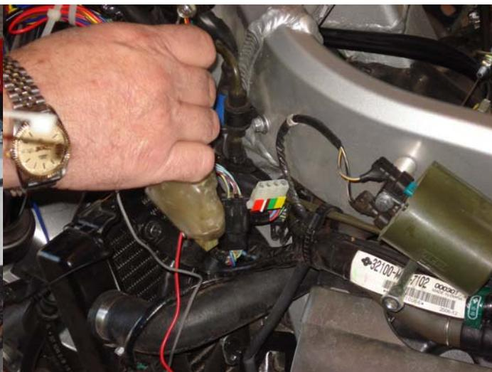
20. The control head was mounted on the handlebars, with the wires routed down to the mating connector. The control head wires were placed in the connector housing, and the connectors were mated.
