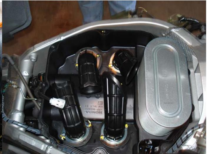
2. The air filter and snorkels are removed. Each one of the 'snorkel' screws has a tab covering the head. Carefully bend the tab up to expose the screw head and remove the screws. The snorkels have stamped index marks – for proper orientation, these marks must be aligned when re-installing. The index marks are circled in red. Once the snorkels are removed, place something in the throttle body intakes to prevent accidentally dropping something in there (white rags were used here).
