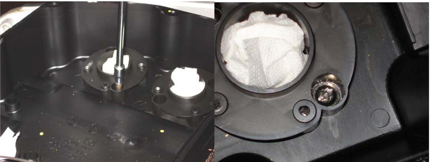
4. The offending air box screw had to be extracted with a drill bit and easy-out. After all the screws are removed, it is a good idea to vacuum the bottom of the air box to rid of bug residue, etc. before removing.
