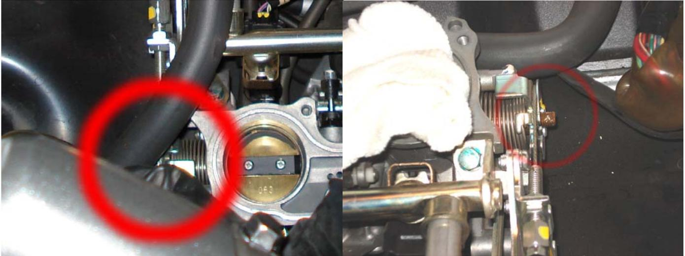
9. Install the lever and washer for the cruise control on the throttle drum. You may want to radius the top corners of the bracket for piece of mind. Later, during the re-install we thought the bracket was chaffing against the crankcase breather hose. The bracket was removed and the corners were rounded off. We later discovered the corners probably did not need to be rounded off, but it was a good piece of mind anyway.
