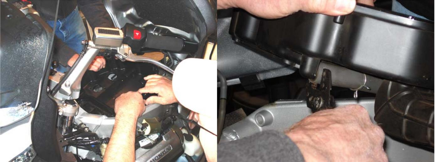
7. Keep track of the small cable clamps on the hoses. It might be a good idea to remove the clamps completely and set aside. The cable clamp on the rear hose initially slipped and fell down on the hose. Later, it must have fallen off completely as it could not be located – another clamp had to be located during the re-install.
