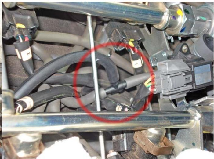
16. A check valve is installed on the Audiovox vacuum line. The diameters on the stems of the check valve were different than the vacuum hose, so an additional coupling and hose was added along with a dab of RTV silicone.
