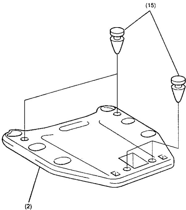
5. Install the rear carrier base on the motorcycle as shown.
