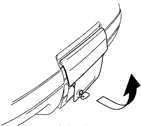
3. Pull the plate lock down. The lid can now be opened and closed.
