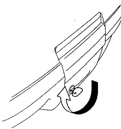
2. With the key turned clockwise, pull the plate lock out toward you, then pull it up in the direction shown.
