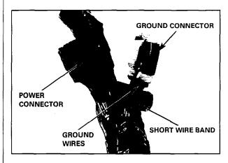
5. Use the large wire band to secure the ground connector, power connector, and wire harness together.
