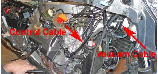
15. The Audiovox vacuum line needs to be tied into the vacuum on the ST1300. There are several places the vacuum could be obtained. During this install, the vacuum line to the MAP sensor was cut and a Tee was installed for the Audiovox vacuum.
