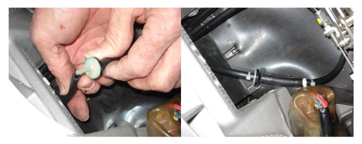
17. The control cable is connected to the bracket, and then connected to the lever via the chain. Shrink tubing is added over the coupling between the ball at the end of the cable and the chain.
