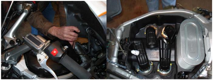
2. The air filter and snorkels are removed. Each one of the 'snorkel' screws has a tab covering the head. Carefully bend the tab up to expose the screw head and remove the screws. The snorkels have stamped index marks – for proper orientation, these marks must be aligned when re-installing. The index marks are circled in red. Once the snorkels are removed, place something in the throttle body intakes to prevent accidentally dropping something in there (white rags were used here).
