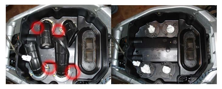
3. The lower portion of the air box is removed. The eight (8) screws attach thru the round snorkel bases, lower portion of the air box, and into the throttle bodies. The round snorkel bases are identical; however, it is good to take note of the orientation of the bases so that the same screw holes for the snorkels can be utilized when re-installing on the bases.
