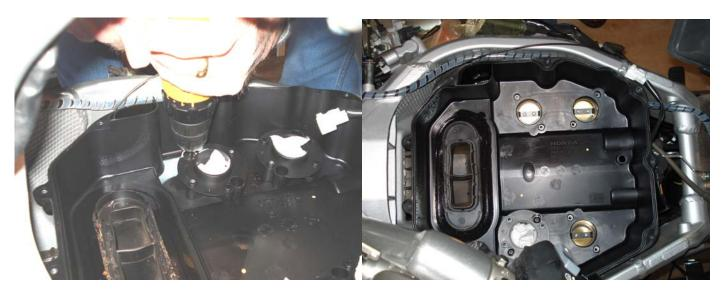
5. A check of the extracted screw shows signs of galvanic corrosion (white powdery appearance). A comparison between the extracted screw and an adjacent screw shows the difference. As you can see, there is ample room to drill and use an extractor if you find yourself in this situation. Luckily, Fred had a brand new replacement screw handy.
