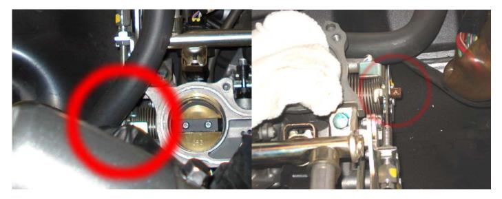
9. Install the lever and washer for the cruise control on the throttle drum. You may want to radius the top corners of the bracket for piece of mind. Later, during the re-install we thought the bracket was chaffing against the crankcase breather hose. The bracket was removed and the corners were rounded off. We later discovered the corners probably did not need to be rounded off, but it was a good piece of mind anyway.
