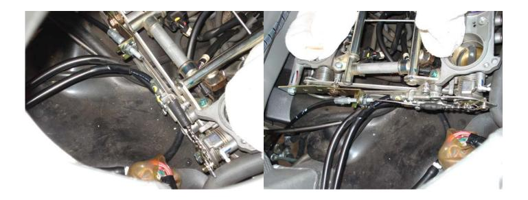
18. The Violet wire from the Audiovox cruise control is connected the Green/Yellow wire from the Red connector on the front right side of the bike. The Green/Yellow wire is on the rear (left) half of the Red connector. The wire was extracted from the connector and the Violet wire was soldered to it, and covered with shrink wrap.
