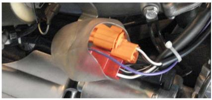
19. Power wires on the Audiovox cruise control were wired up. Power was tapped from the Quartet harness, with the in-line fuse routed to the proximity of the main fuse box for easy access. Slack in the wires was taken up with tie wraps. The pins were placed in the appropriate color coded connector housing.
