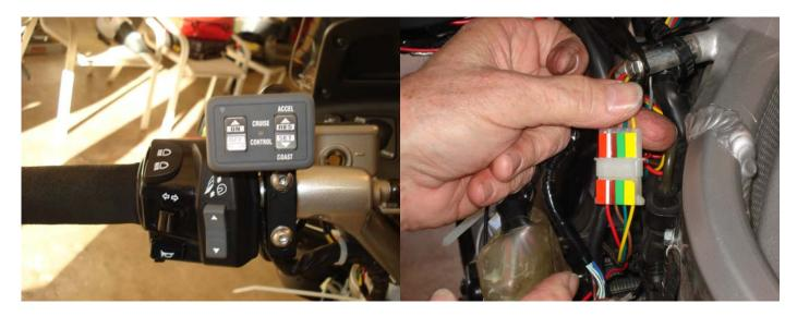
21. The blue wire was connected to the ignition coil, and the ground wires were connected to the frame.
