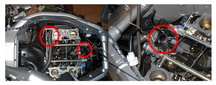
8. The lever for the Audiovox cruise control is installed on the throttle drum, which is attached to the throttle body. The throttle drum is somewhat masked by the crankcase breather hose in the first picture. The second picture is a close up of the throttle drum with the nut removed. Page 5-65 of the service manual also shows a picture of the throttle drum.
