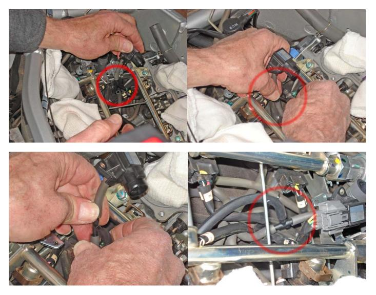
16. A check valve is installed on the Audiovox vacuum line. The diameters on the stems of the check valve were different than the vacuum hose, so an additional coupling and hose was added along with a dab of RTV silicone.
