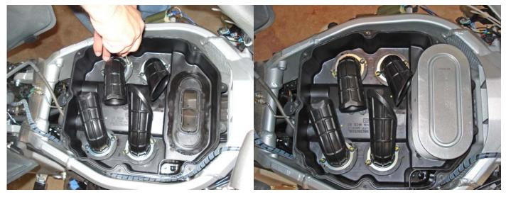
23. The top portion of the air box, IAT sensor cable, and tank ground cable is re-installed. The tank is re-installed.
