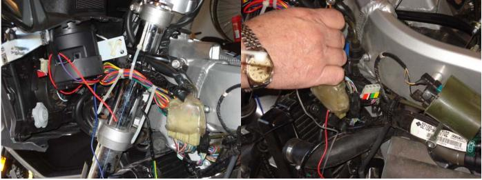
20. The control head was mounted on the handlebars, with the wires routed down to the mating connector. The control head wires were placed in the connector housing, and the connectors were mated.
