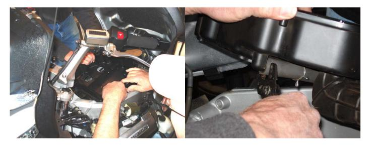
7. Keep track of the small cable clamps on the hoses. It might be a good idea to remove the clamps completely and set aside. The cable clamp on the rear hose initially slipped and fell down on the hose. Later, it must have fallen off completely as it could not be located – another clamp had to be located during the re-install.
