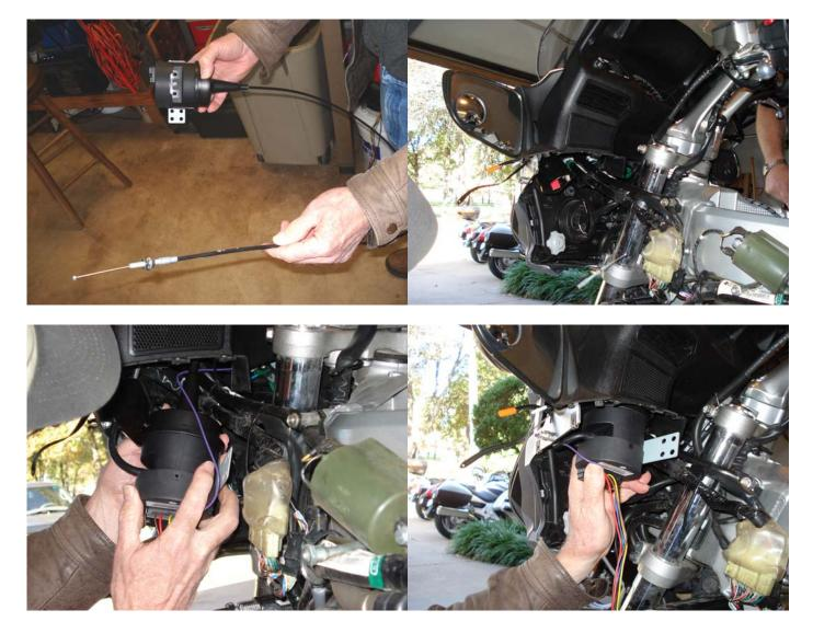
13. Zip ties were used to attach the control box the bike. Dry fit the panels to ensure there are not clearance issues.
