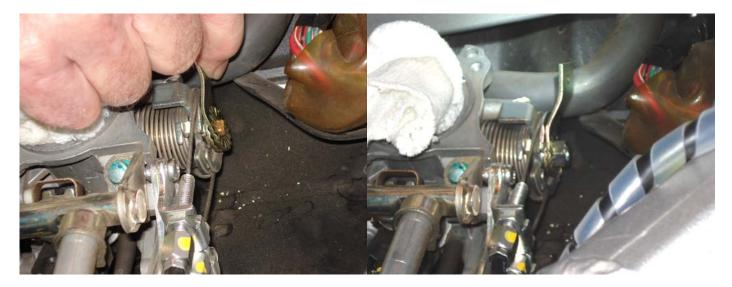
10. Install the opposing Audiovox bracket on the throttle body. One screw will need to be removed and re-installed thru the bracket.
