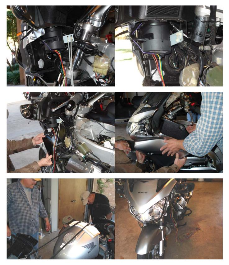
14. Route the vacuum and control lines to the throttle body. This step may take some time to find the optimal locations where no kinking or binding will occur. A nice sweeping radius is needed for the control cable.
