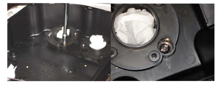
4. The offending air box screw had to be extracted with a drill bit and easy-out. After all the screws are removed, it is a good idea to vacuum the bottom of the air box to rid of bug residue, etc. before removing.
